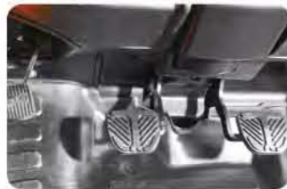
Foot operated park brake offering easy and safe engagement.
