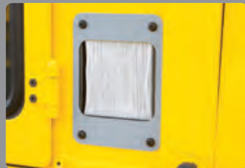
Cabin air fresh filter The internal pressure is maintained to be slightly higher than that of outside to exclude dust and to reduce noise levels.
